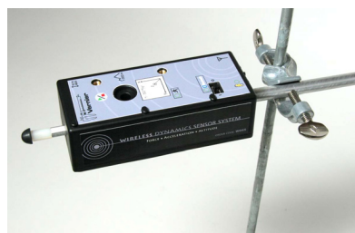
WDSS with rod threaded into the end
